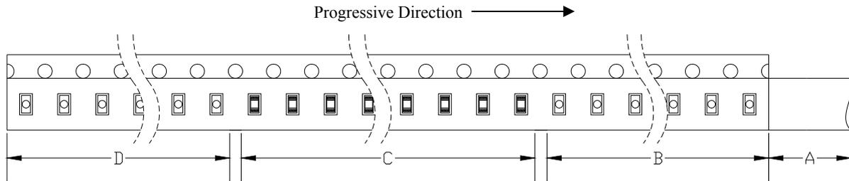
A: Top Cover Tape, 300mm; B: Leader, Empty, 200mm; C: 3000 Lamps Loaded; D: Trailer, Empty, 200mm.
