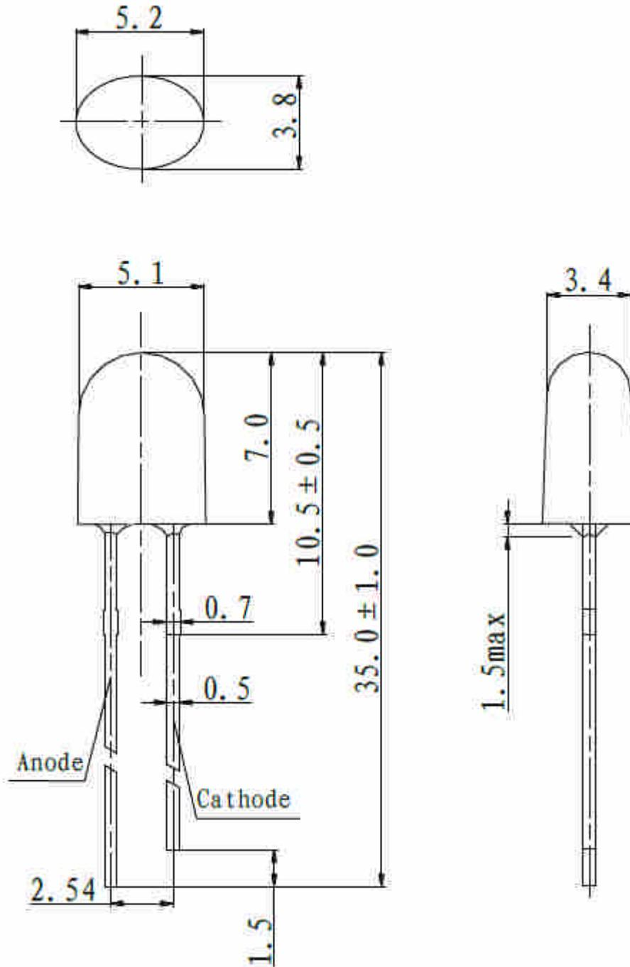
All dimensions in mm, tolerances unless mentioned is  $\pm 0.2$  mm.
