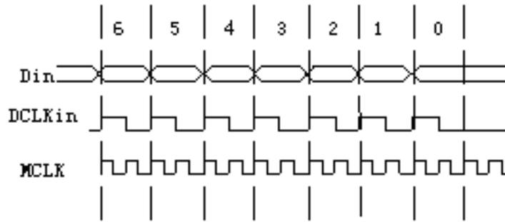
Figure 3: Timing of Clock latched mode signals
