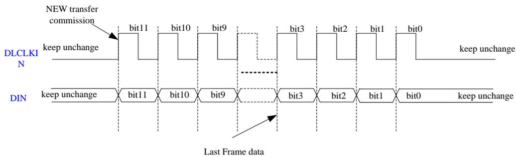
Figure 4: General serial data timing relationship
