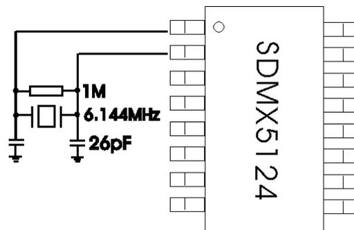
Figure 2: Oscillator configuration
