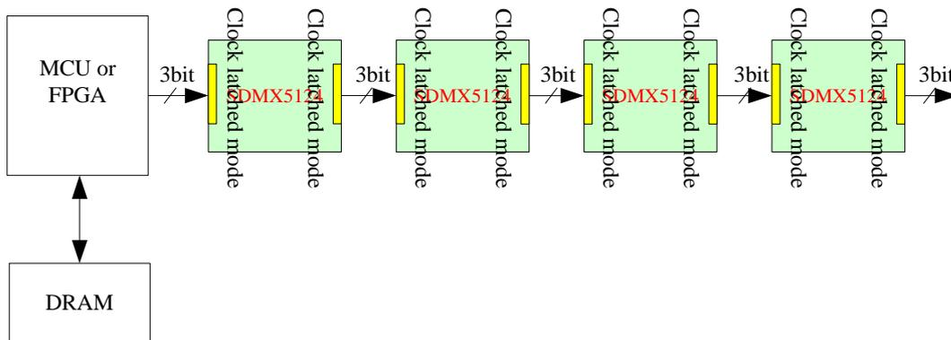
Figure 5: Clock latched mode chain
