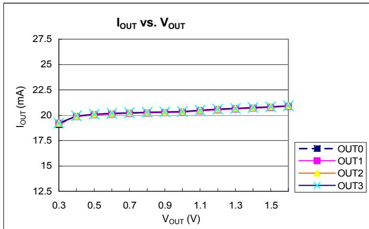
Fig. 1 (@  $V_{LED} = 7.5V$ ,  $T_a = 25^\circ C$ )
