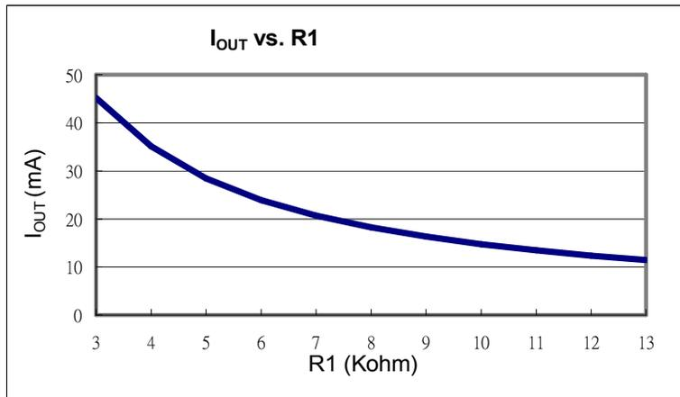
Fig. 2 (@  $V_{LED} = 7.5V$ ,  $T_a = 25^\circ C$ )
