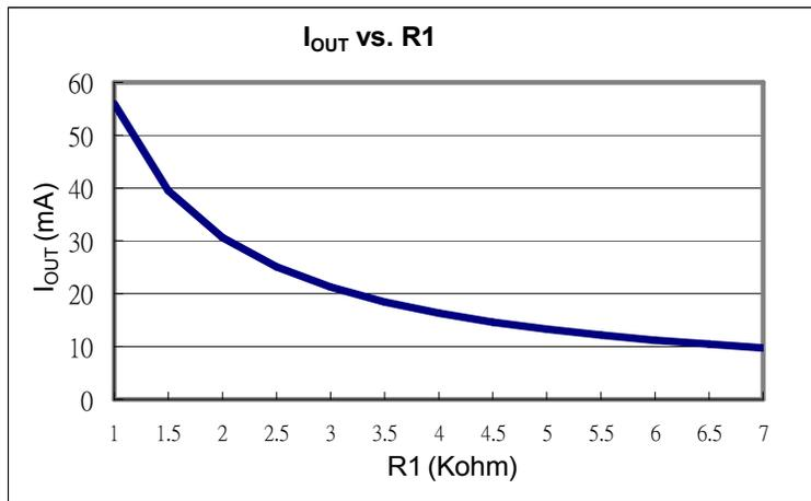
Fig. 4 (@  $V_{LED} = 4V$ ,  $T_a = 25^\circ C$ )
