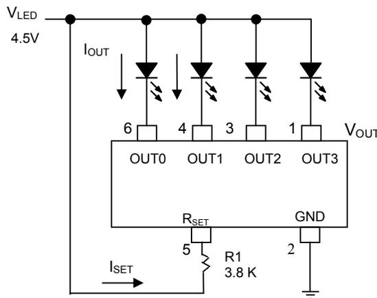
※Neither a capacitor, an inductor nor Schottky diode is needed.
