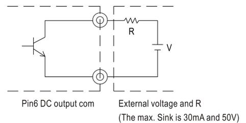
Fig 2.2 Internal circuit of AC OK (Battery Low)
