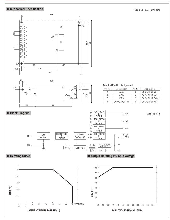
65W Quad Output Switching Power Supply
