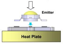
Put Emitter on MCPCB. Take the MCPCB out from Heat Plate within 10 seconds.
