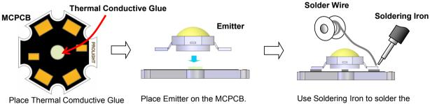
Use Soldering Iron to solder the leads of Emtter within 5 seconds.
