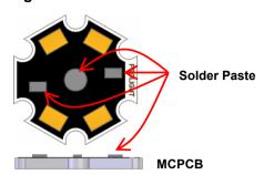
Use Solder Mask to print Solder Paste on MCPCB.
