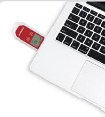
Connect the logger to computer and configure parameters accordingly
