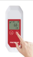
Press and hold the START button for 3 seconds to start recording, the screen will flash the characters of go.
