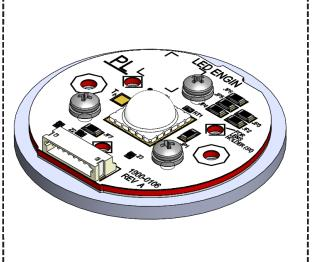
Mounting structure (exploded view)
