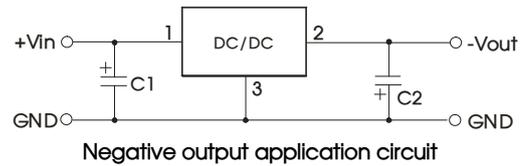
Fig. 2 Typical application circuit
