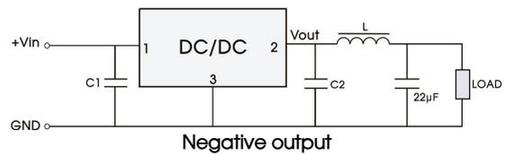
Fig. 4 "LC" output filter application
