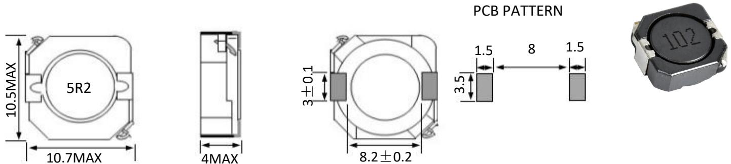
**● Packing method and dimension and Printing Direction(Unit:mm)**
