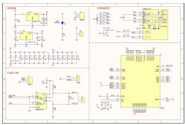
TXD1 and RXD1 are compatible with 3.3V and 5V level, and the RS485 control pin DIR can be suspended if not used.
