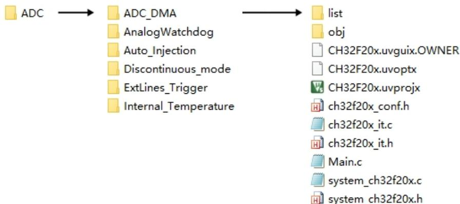
As shown above, "ADC" means ADC basic function demo, double click in this folder to open the project "
