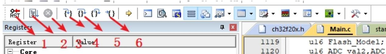
1-Reset: Its function is equivalent to the reset button on the hardware, the code will be executed again from the beginning after pressing it once.
