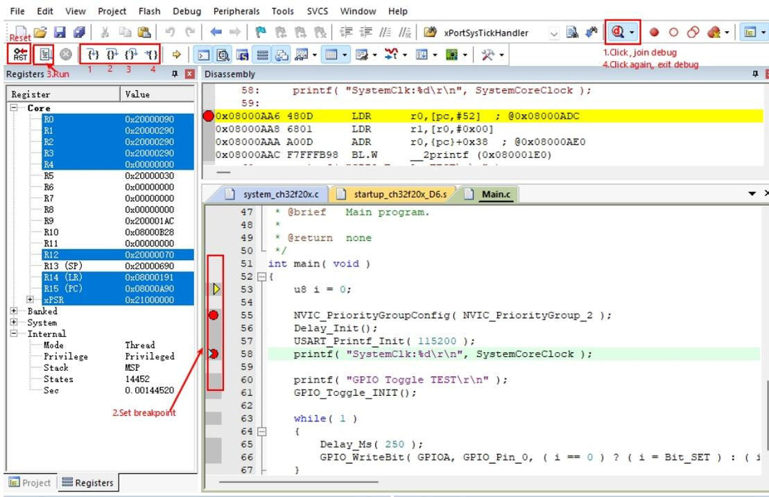
Take the ADC\_DMA program in EVT as an example, single-step debugging is applied, the debugging position is displayed by cursor, and the serial assistant is applied to view the result. The result of single-step operation is shown in the figure below.
