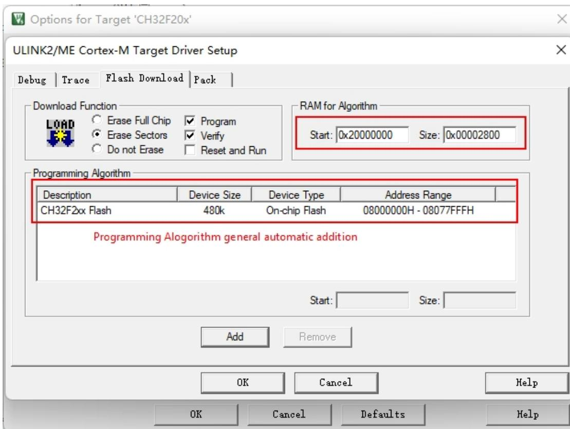
Note: When you select the algorithm file, you need to fill in the size of RAM for Algorithm as 0x2800.
