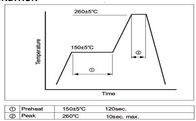
Total time 200sec. max. Solder melting point: 185°C
