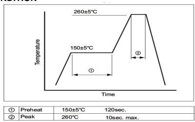
Total time 200sec. max. Solder melting point: 185°C
