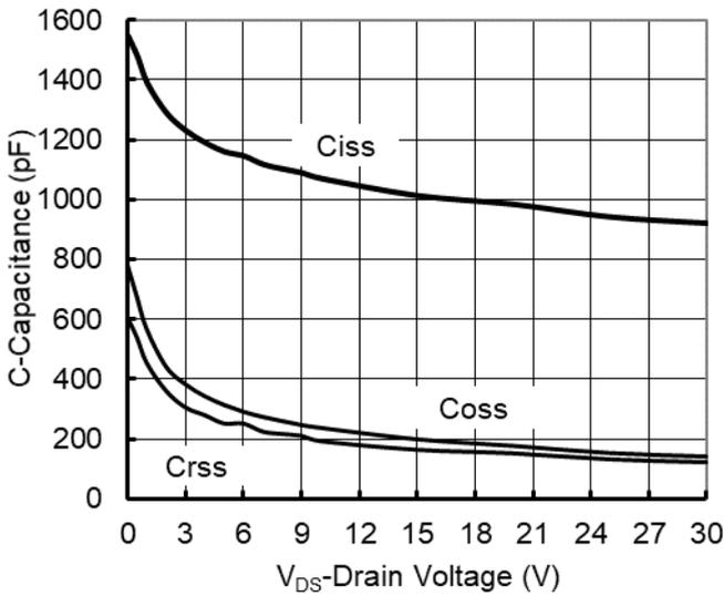
Figure 3. Capacitance Characteristics
