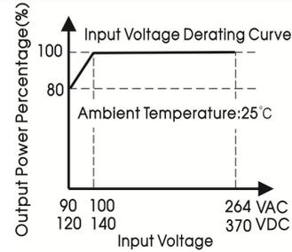
Note: 1. With an AC input voltage between 90 -100VAC and a DC input between 120-140VDC the output power must be derated as per the temperature derating curves;
