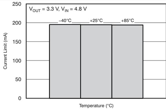
Figure 9. Current Limit vs Junction Temperature
