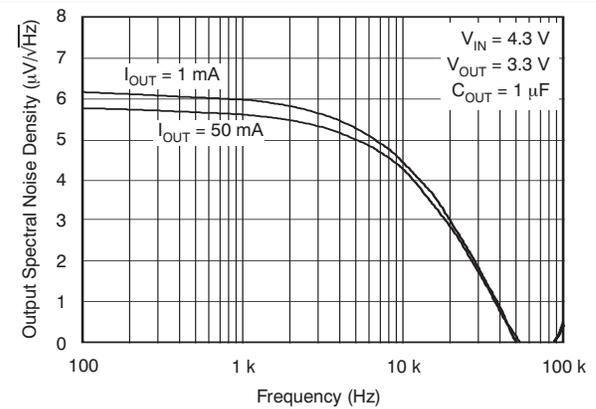
Figure 10. Output Spectral Noise Density vs Frequency
