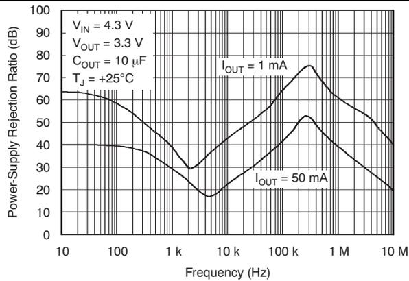
Figure 11. Power-Supply Ripple Rejection vs Frequency
