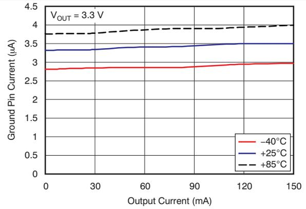
Figure 8. Ground Pin Current vs Load Current
