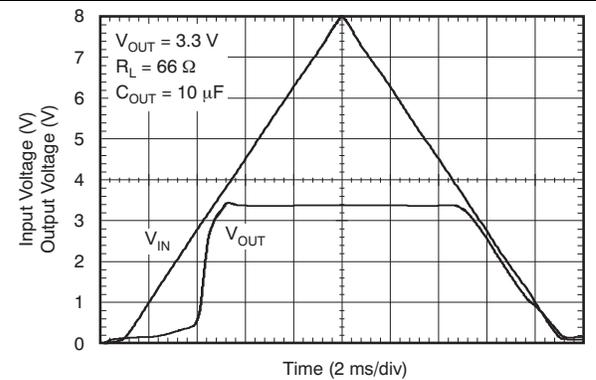
Figure 12. Power Up/Power Down
