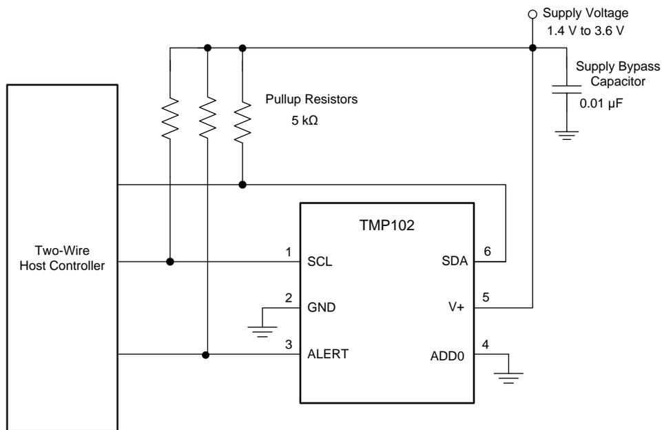
**Figure 14. Typical Connections**
