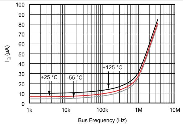
Figure 4. Quiescent Current vs Bus Frequency (Temperature at 3.3-V Supply)
