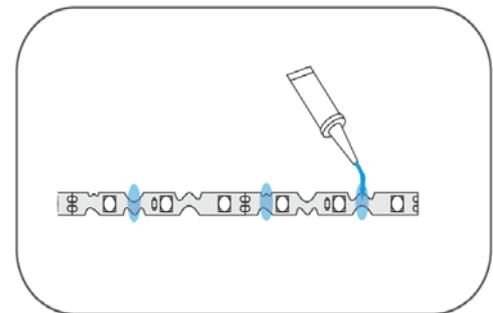
After installing the LED strip, LED strip surface is glued once again to reinforce the LED strip on the board at least every 10cm so as to prevent the LED strip from detaching. Note that glue cannot be coated on the LEDs.
