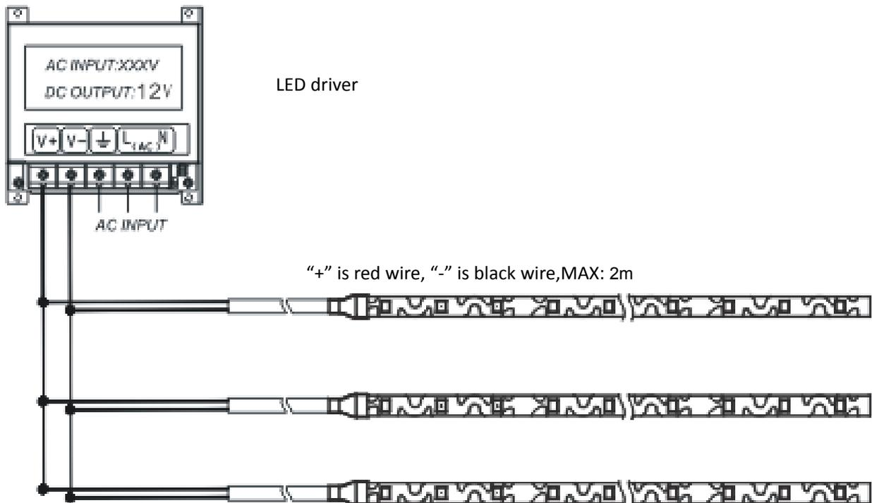
(Note: Please connect the '+' and '-' of wires to those of power supply output correctly.)
