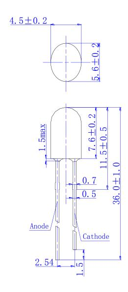
All dimensions in mm, tolerances unless mentioned is  $\pm 0.2$  mm.
