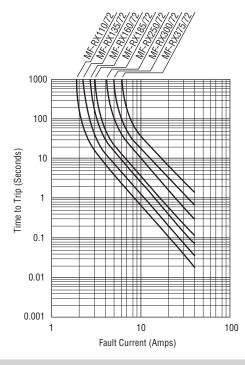
The Time to Trip curves represent typical performance of a device in a simulated application environment. Actual performance in specific customer applications may differ from these values due to the influence of other variables.
