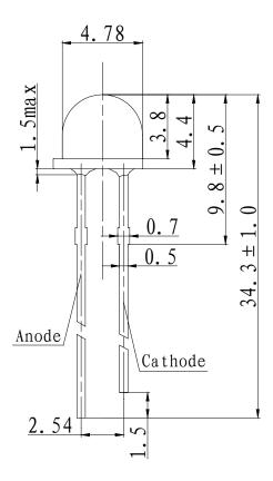
All dimensions in mm, tolerances unless mentioned is  $\pm 0.2$  mm.
